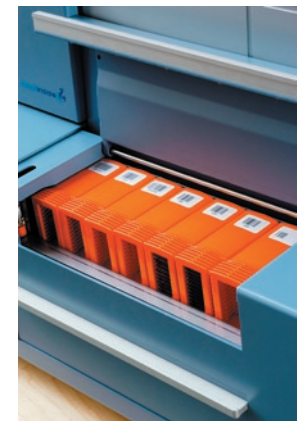
Slides are placed into a 12-position magazine; up to 8 magazines, containing a total of 96 slides, can be loaded at once.
